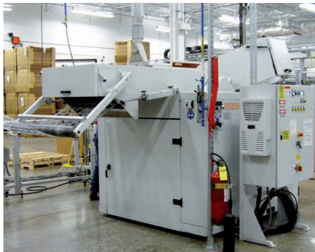
图1: RS 4500系列大型造粒机,设计产量可高达1500 kg/h。 图片所示设备的型号为RS 4509 Image 1: The large granulators of the RS 4500 model series are designed for throughputs up to 1500 kg/h. The photo shows an RS 4509-E (Photos: Getecha)
