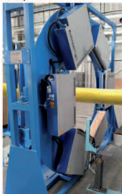
3-axis ODAC® 550 measuring system for Ø up to 500 mm
