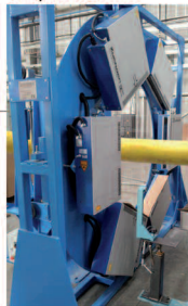
3-axis ODAC® 550 measuring system for Ø up to 500 mm
