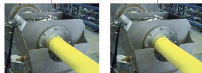
UMAC® scanners with 8 measuring points for Ø up to 690 mm (bigger on request)
