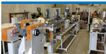
Filament production line for 3D-Printer Extruder up to 20mm
