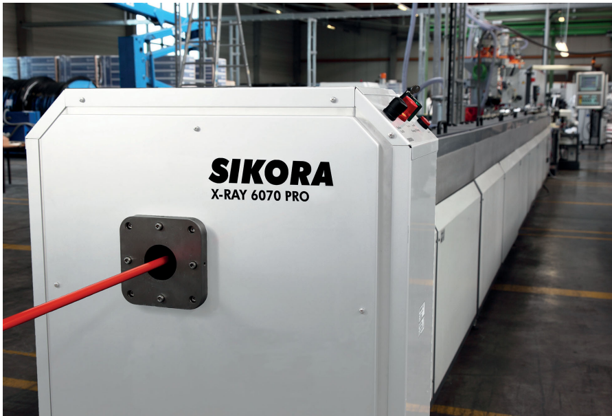
Pic. 4: X-ray measuring system installed in a hose extrusion line
