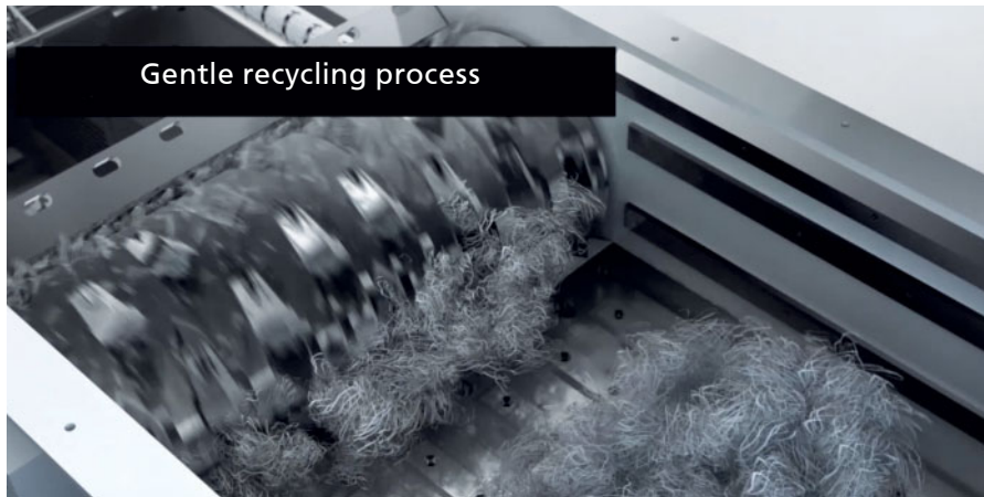
Picture 3: Instead of using an agglomerator or a cutter-compactor which processes the material at a higher temperature for a longer period of time, the gentle yet powerful single shaft shredder cuts the raffia waste within a short time at a much lower processing temperature. This helps to maintain the property of the post-industrial waste material as close to new material as possible
