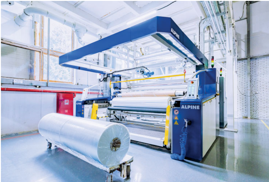
Film Winder by Hosokawa Alpine, installed at Grand-Master, Russia
