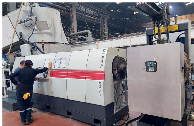
The Starlinger C-VAC degassing module increases the melt surface by 300 %, thus achieving an extremely high degassing efficiency (Pictures ©Starlinger)
