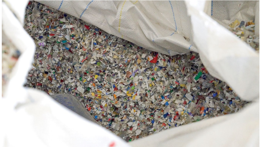
Figure 2: Blend of PP flakes (PCR)
