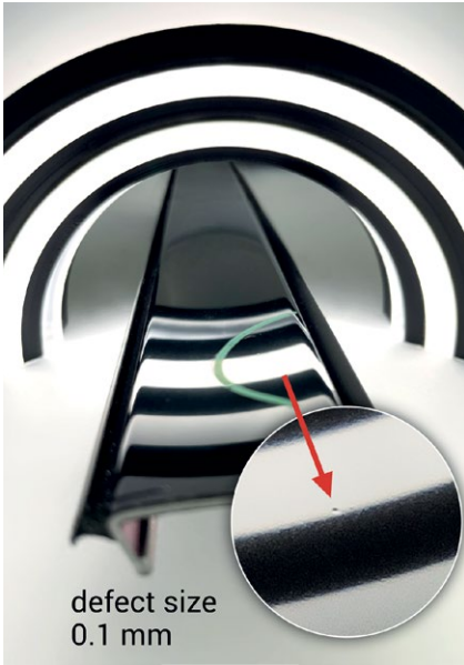
The PIXARGUS Shiny Detection module casts a pattern of structured light onto the high-gloss surfaces of the profiles to be inspected. These light patterns showing on the surface of the profile allow even extremely small scratches, bubbles or dents to be reliably detected (Photo ©PIXARGUS)
