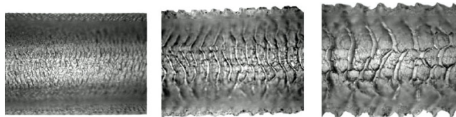
Magnified View of Melt-Fractured Surface
