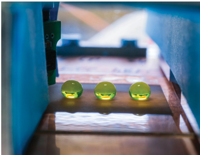
Fraunhofer scientists study how anti-icing coatings affect the freezing behavior of water droplets in an icing chamber (© Photo Fraunhofer IVV)
