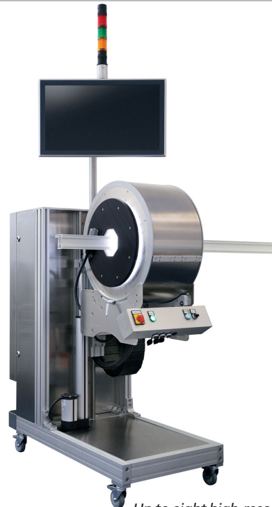
Up to eight high-resolution GigE CMOS cameras measure the inner cross-section geometry of profiles of up to 250 mm diameter. In combination with an upstream installed DualVision system, it is even possible to inspect surface defects and the outside contour in parallel. (Source: PIXARGUS)
