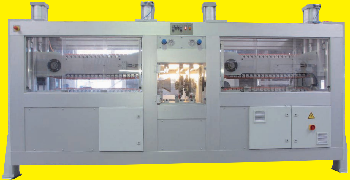
"PCL" separation combination: feeder (right), blade unit (centre) with several replaceable cutting blades, haul-off unit (left). The caterpillar pairs are fitted with standard pads like the ones generally used in profile production.
