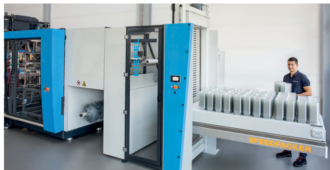
SpeedPacker - Buffer and Unloading Station for KMD Speedformer Series
