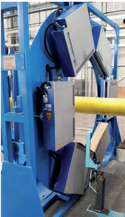
3-axis ODAC 550 system, measuring an Offshore cable of 500 mm OD
