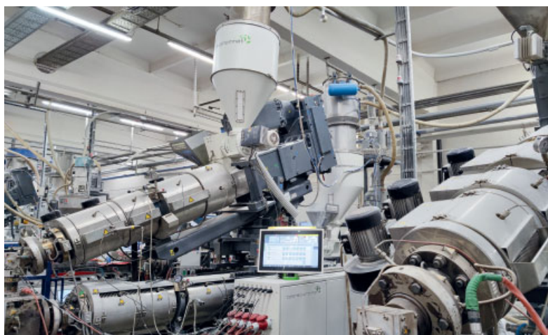
Coextrusion with twinEX 78-34 as the main extruder, combined with a conEX NG 65 as co-extruder
