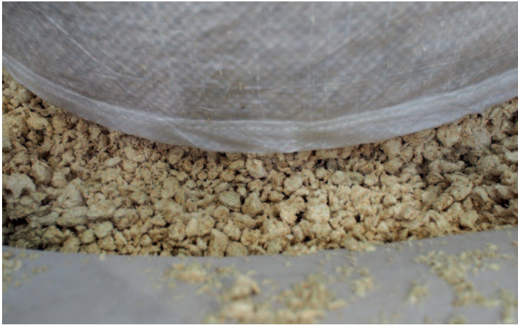
The formulation had an extremely low bulk density of 270 g/l and was processed in the form of an agglomerate
