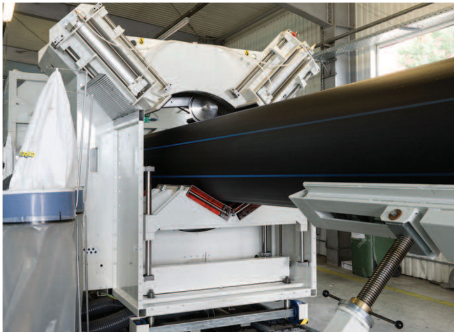
The cutStream PTA 1200 cutting tool can cut both swarfless or with swarfs, depending on the application (all images © Tehno World)
