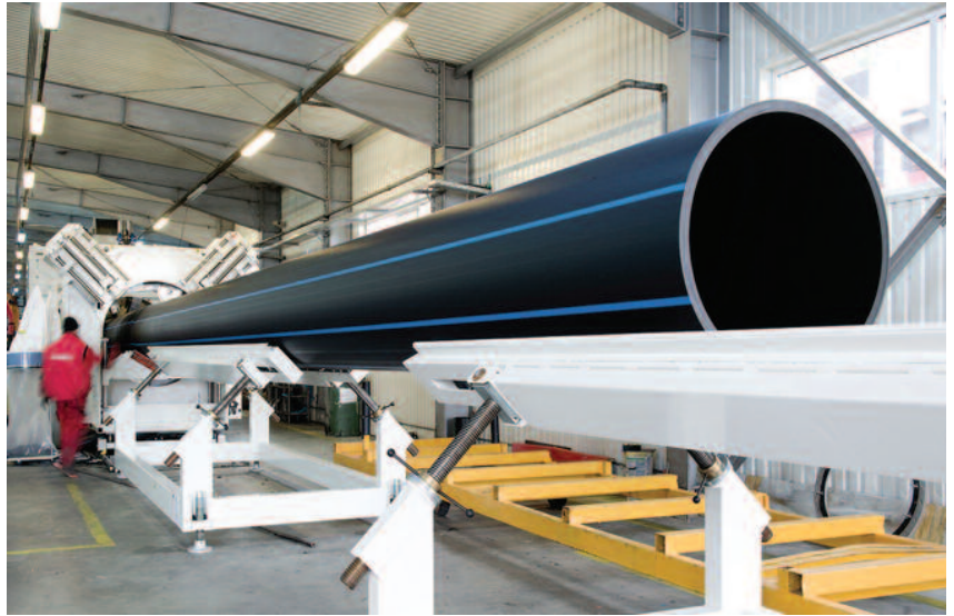
A 1.2 m pipe with color stripes produced on the battenfeld-cincinnati line
