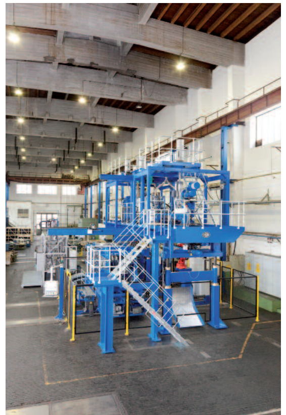
Large machine construction in Traismauer: Final assembly in Traismauer of a 6-layer tank system blow moulding machine, type BA 220 M Coex, for the automotive sector
