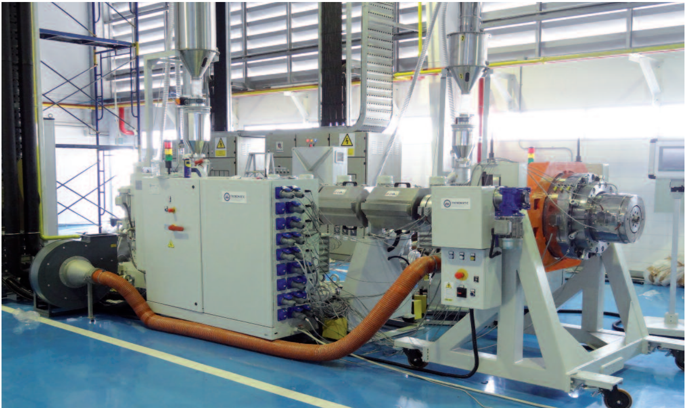
VEGA extruder 75.37 with VENUS 400 and PAC air cooling system, for efficient pipe production
