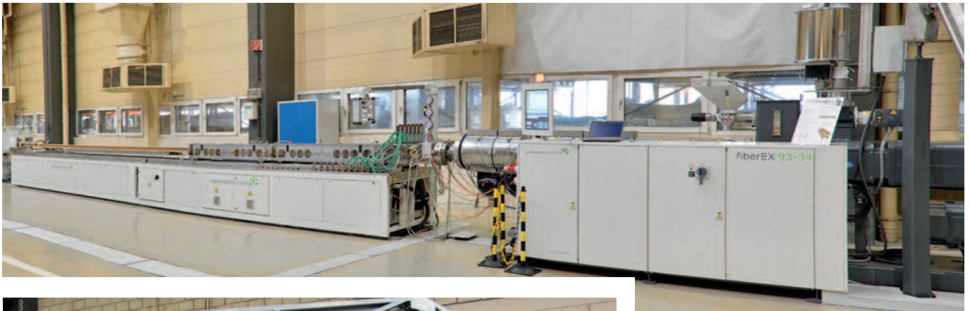
The extrusion line with the fiberEX 93-34D extruder, on which an H profile was produced
