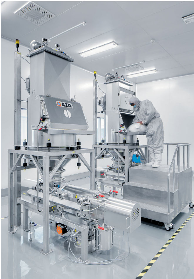
Easy to clean cyclone screener type DA 650 with extraction device
