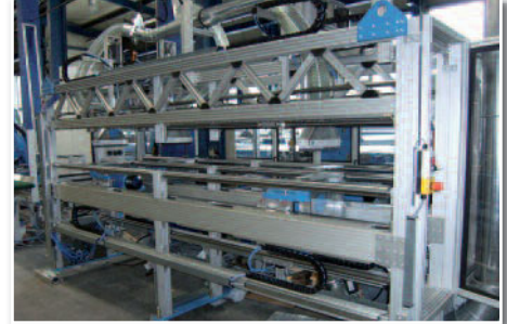
Slitting RB 2 with four sawing stations
