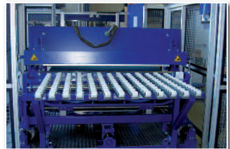
Transverse separating cutter QSS, inlet
