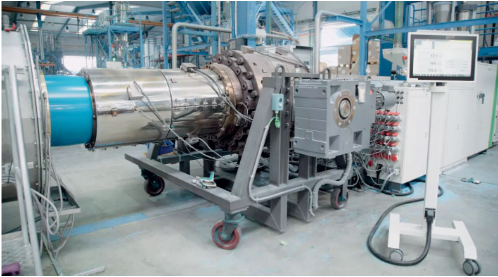
Twin screw extruder twinEx for the extrusion of O-PVC pipes
