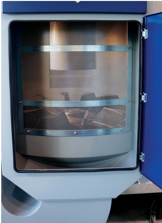
Picture 5: Detail view through a tangential sieve into the centrifuge chamber of the DRD 26 system. Below the double rotor system with 12 rotor blades, above the heating register housing (Photo: Author)
