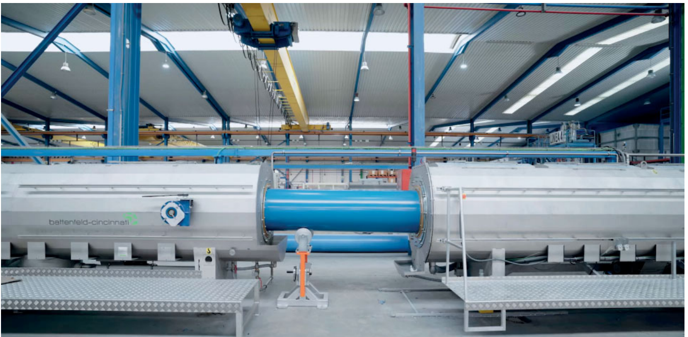
PVC-O pipe extrusionsline - vacuum bath
