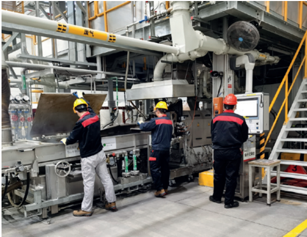
Commissioning of the KraussMaffei compounding line at Lanxess' Chinese production site in Changzhou has now been completed
