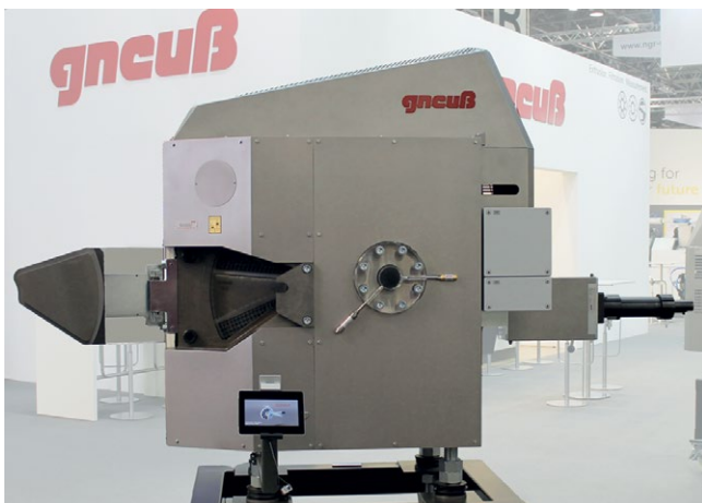
RSFgenius Filtration System 330 for LDPE/LLDPE Film Recycling
