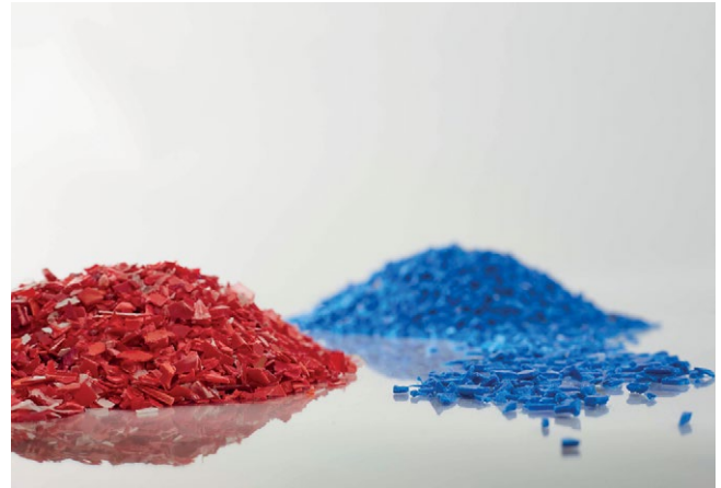
Sensor-based sorting accurately separates red and blue PP flakes
