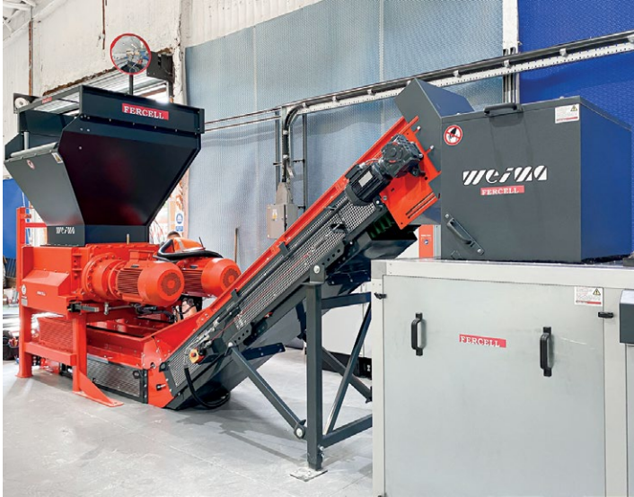
Two-stage shredding for Plastipack with WEIMA shredders
