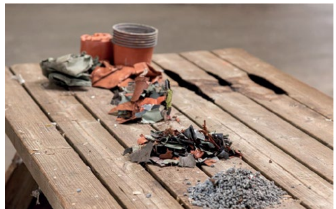
Flower pot recycling cycle: raw material, flakes, & granules
