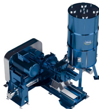
The HV 70 plastcompactor is the most powerful of the series from Herbold Meckesheim. It processes the feedstock in continuous operation between a rotating and a fixed compactor disk, which are equipped with screwed-on and easily exchangeable kneading bars (Photo: Herbold Meckesheim, Meckesheim, Germany)
