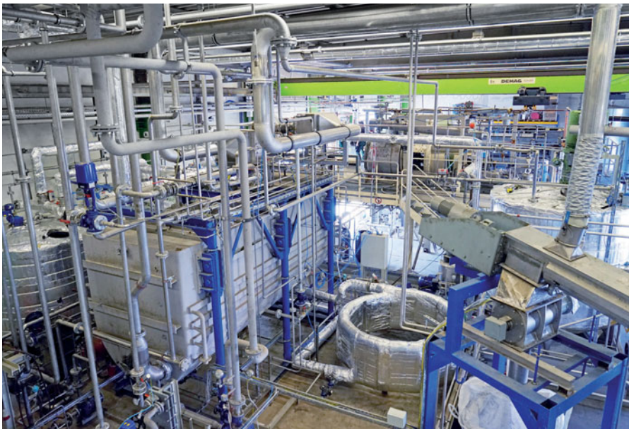
Trenntechnik Ulm GmbH has installed a line specifically for the chemical separation of PA/PE composite films in Memmingen. Using this method and a suitable solvent, it will be possible to recover other raw materials as well. Image: Trenntechnik Ulm
