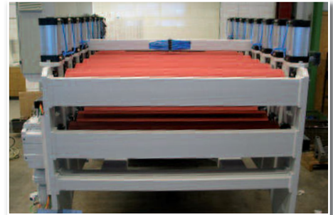
Roller withdrawal AZ 8, outlet side
