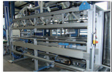
Slitting RB 2 with four sawing stations
