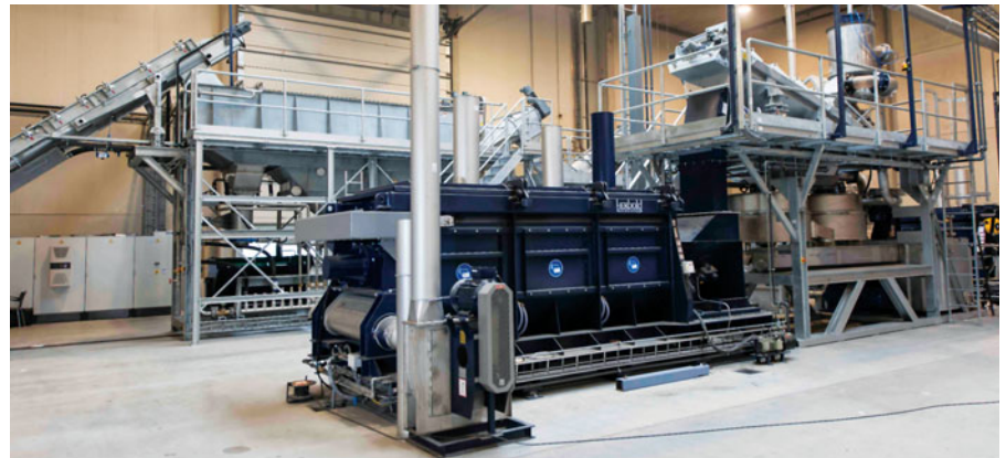
Pic. 3: Hydro cyclone and Dryer, in the background Pre-washing unit
