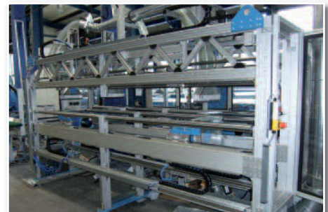
Slitting RB 2 with four sawing stations
