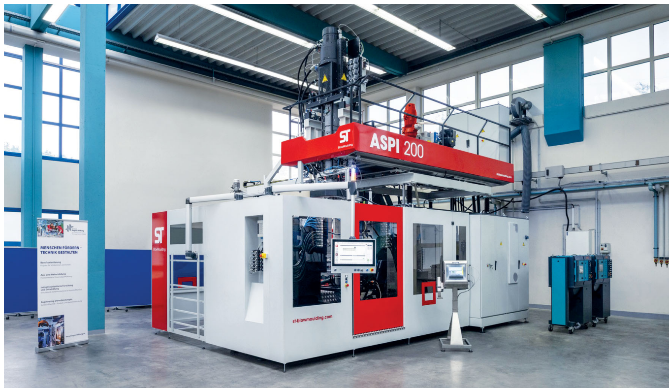
The ASPI 200 is suitable for both suction blowing (3D) and conventional blow molding (2D)
