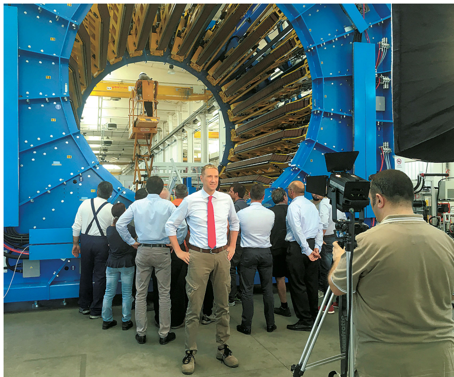
P3500/24 Plus multi-caterpillar haul-off for pipes up to pipes up to 3.5 m (138 in.)
