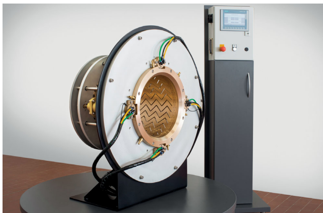
CCA's latest innovation: The motor-controlled calibration sleeve for controlling the diameter and the ovality of the pipe (inline). Designed for plastic pipes from 280 up to 2600 mm (also available in inch sizes)
