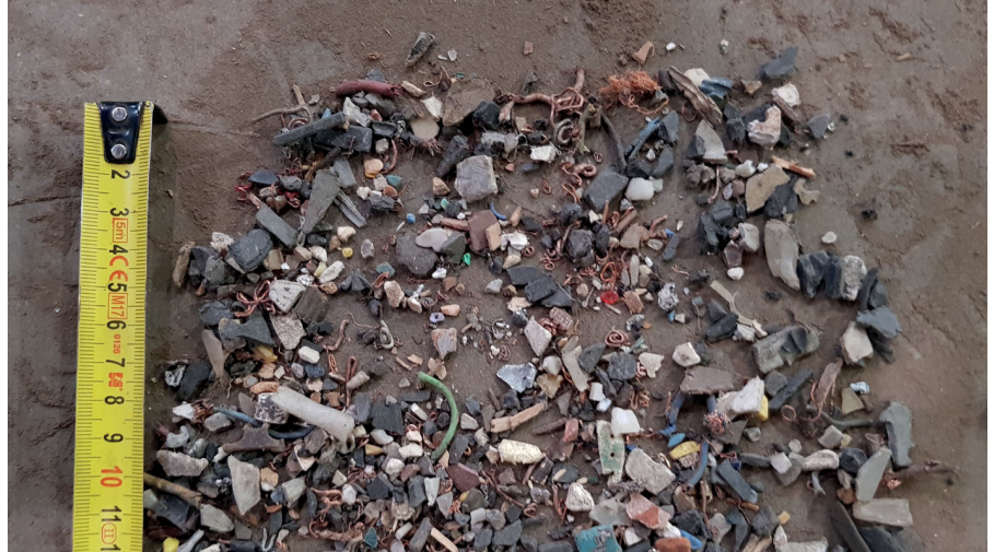
Optimal pelletizing is being carried out on valuable copper components in the rotor impact mill
