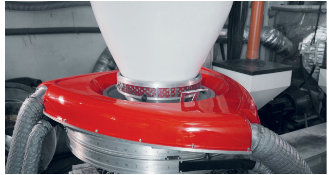
Film thickness control system
