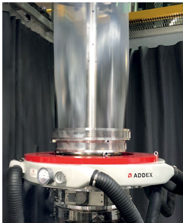
Short Stack trials running 90% 1MI LLDPE rich blend demonstrate a 28% increase in output over Addex’s original Intensive Cooling™ “Down-on-the-Die” version, which already improves output by 10 to 15% over conventional dual-flow air rings
