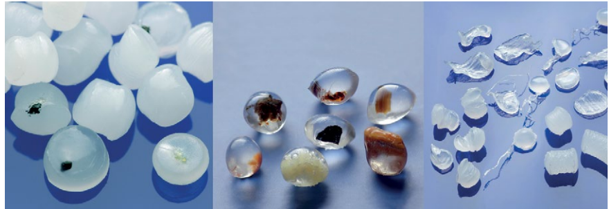
Inspectable contaminations as well as measurable size & shape changes on pellets
