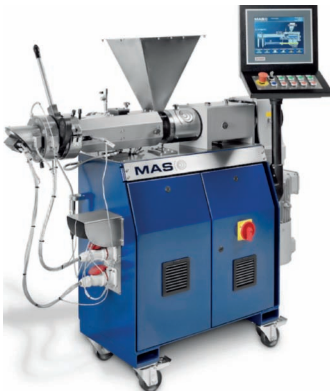
Fig. 1: The lab version of the conical co-rotating twin-screw extruder type MAS 24 is characterised by a plasticising unit that is just 400 mm long
