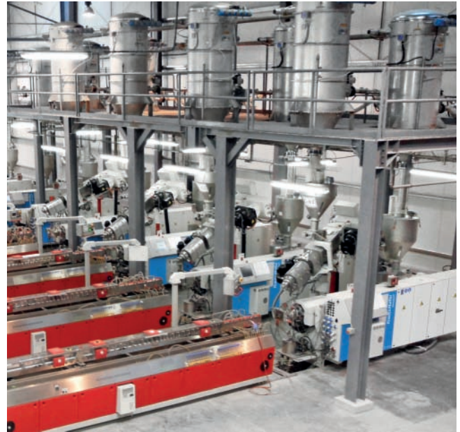
Profile extrusion lines in production
