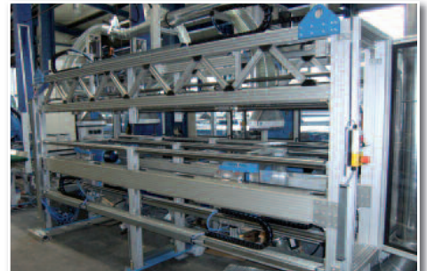
Slitting RB 2 with four sawing stations
