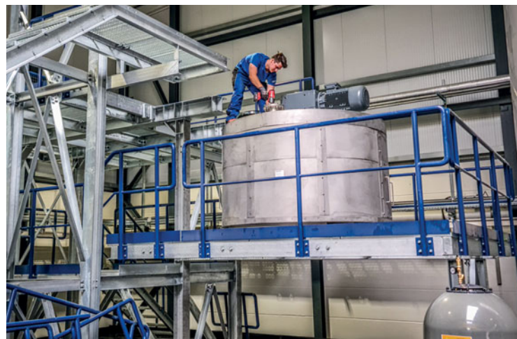
Lindner's new PET hot-wash tower for high-quality PET recycling (Copyright: Linder Recyclingtech)
