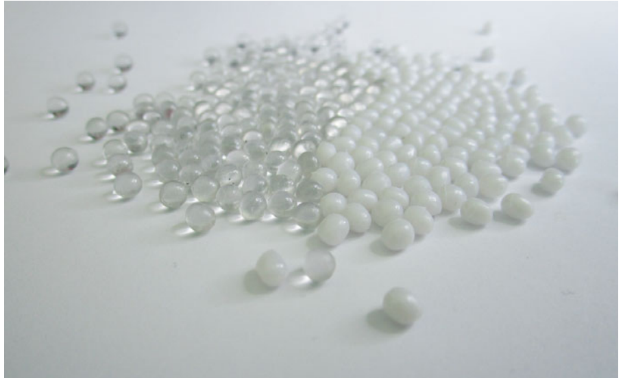
Example of use PET: amorphous pellets on the left, semicrystalline pellets on the right
