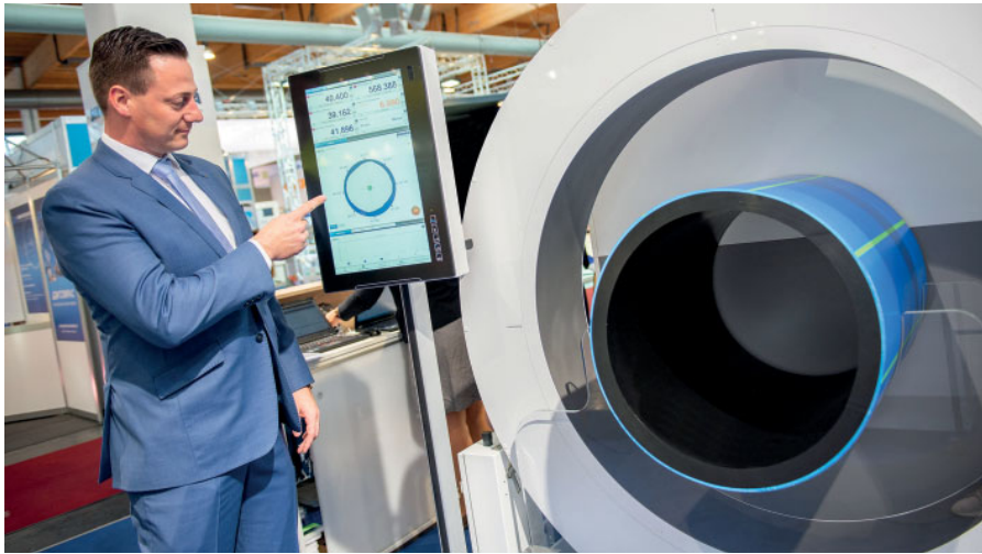
At the Fakuma, SIKORA shows the CENTERWAVE 6000 for quality control during the pipe extrusion
