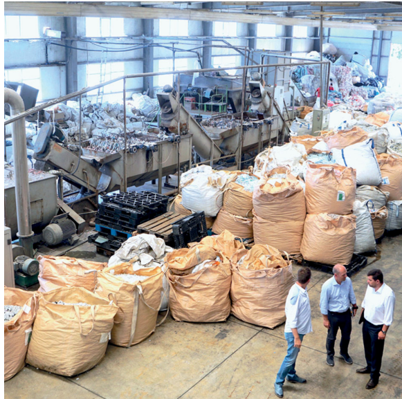
Picture 4: A meticulous material processing by shredding, washing and drying creates the basis for the Kaskada quality granules. There are several preparation lines in operation
