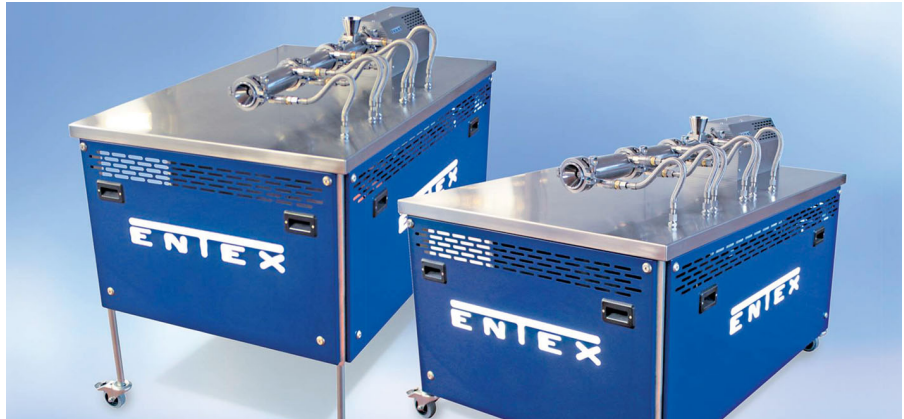
The trade fair exhibit, the L-WE 30 laboratory roller extruder: The height of the lavishly designed base frame can be adjusted to the local conditions with the press of a button. In order to achieve high effectiveness and very short reaction times for tempering, it is possible to integrate heat exchangers that can be supplied with primary energy such as pre-heated water into the base frame. Depending on the conveyed material and process parameters, the throughput rate is about 1-10 kg/h.
