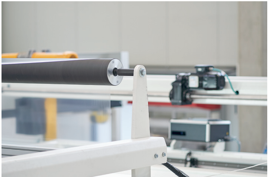
OCS Web Inspection System (FSP600) – Installed OCS camera in film line
