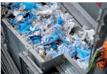
After the bale opening, the films are shredded to an exact size of A4/A3. This enables downstream NIR systems to optimally recognise materials and sort them more efficiently
