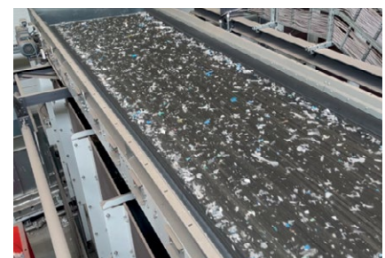
The special shredder set-up of the new Jupiter BW series reduces the proportion of fines that are unusable for the recycler, and which have to be disposed of, by 44%
