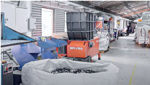
WEIMA WLK 4 single-shaft shredder for plastic scrap at Plásticos Ojara
