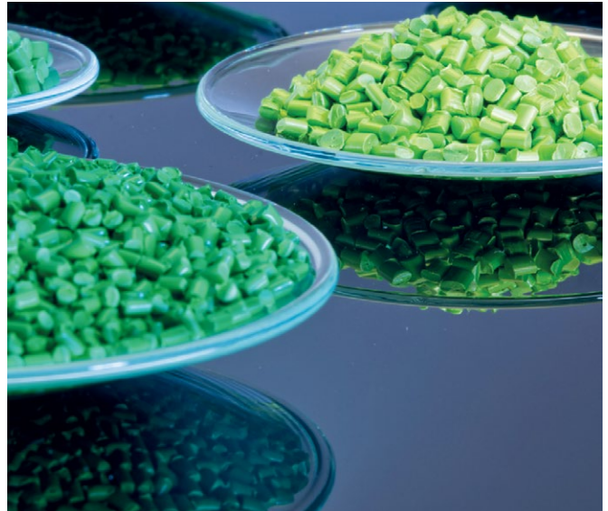
The color masterbatches of the FIBAREC series are based on recycled carrier material and thus ensure sustainability in plastic coloring (Source: Finke)
