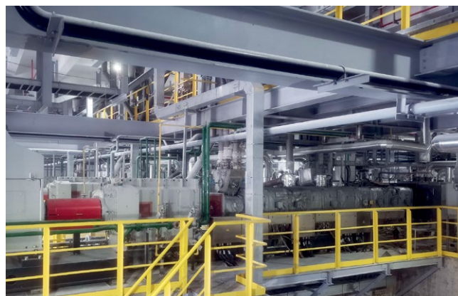
Coperion's ZSK Mc18 twin screw extruder is playing a key central role in this system for particularly energy-efficient manufacturing of acrylonitrile-butadiene-styrene copolymer (ABS) blends (Photo: Zhejiang Zonepic Petrochemical Technology Co., Ltd.)
