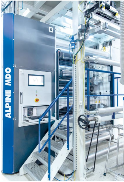
The inline MDO is the centrepiece of the blown film line at Microplast Coldeplast. The monoaxial stretching of blown film improves the film properties and reduces material costs
