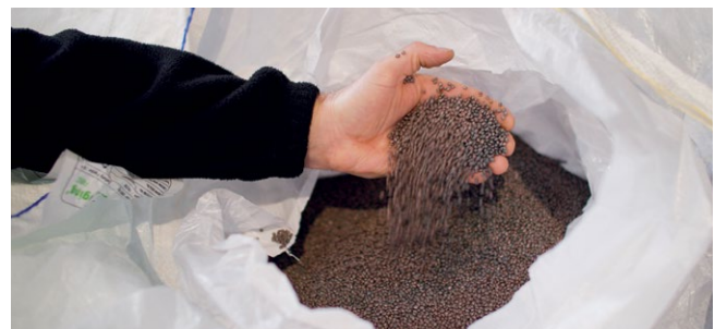
The ISEC evo produces high-quality rPET from used polyester textiles, which can be spun into yarn for use in textiles along with other industrial applications
