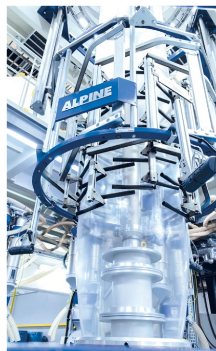
Microplast Coldeplast produces full PE films for various flexible packaging solutions on a 5-layer blown film line from Hosokawa Alpine
