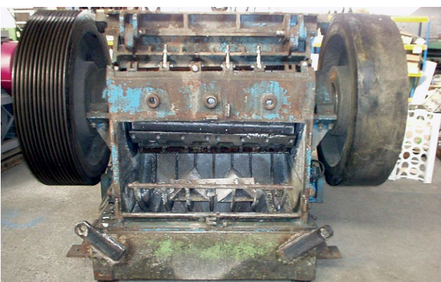
A granulator SMS 80/120 before refurbishment
