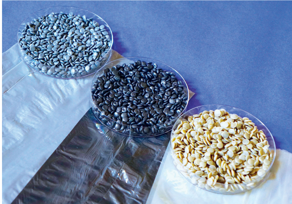
Image 1: The Dutch plastics recycling company DALY Plastics processes 35,000 t of agricultural films and pallet shrink films per year into gray, black and tea-colored polyethylene re-granulates for the reuse in blow film production (All images: TECHNOKOMM)
