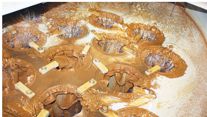
What stays inside these filters cannot harm the production anymore. The load of solids is high in pipe extrusion cooling water – no problem for the Reisner full stream reverse flow filtration system
