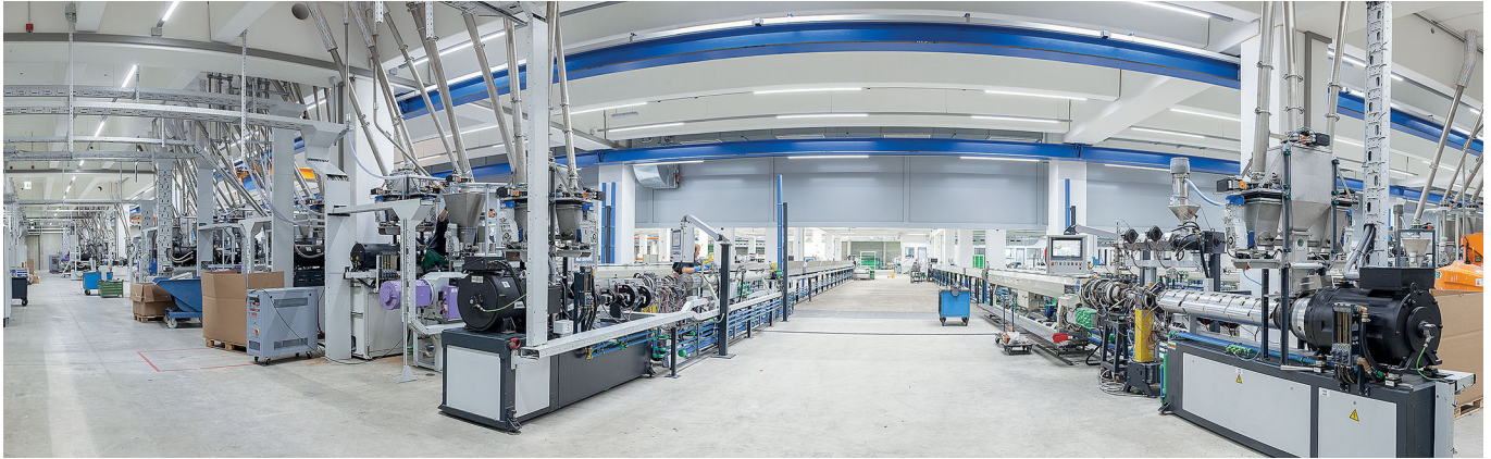
Picture 3: Extrusion facility: aquatherm manufacturers PP-R pipes with diameters of 16 to 630 millimeters (Picture: aquatherm)
