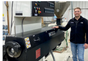
Mark Schnettler with the recent rebuild of a 3.5-inch (90mm) Davis-Standard extruder
