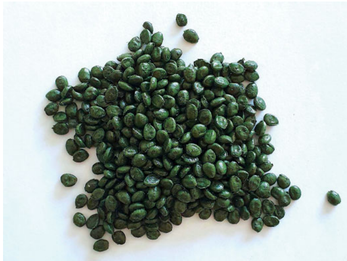
Picture 8: End product of the artificial grass recycling - a high-quality raw material for new quality products (Photo: MAS)
