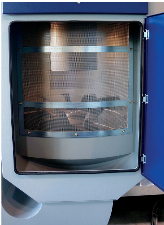
Picture 5: Detail view through a tangential sieve into the centrifuge chamber of the DRD 26 system. Below the double rotor system with 12 rotor blades with 12 rotor blades, above the heating register housing (Photo: Author)
