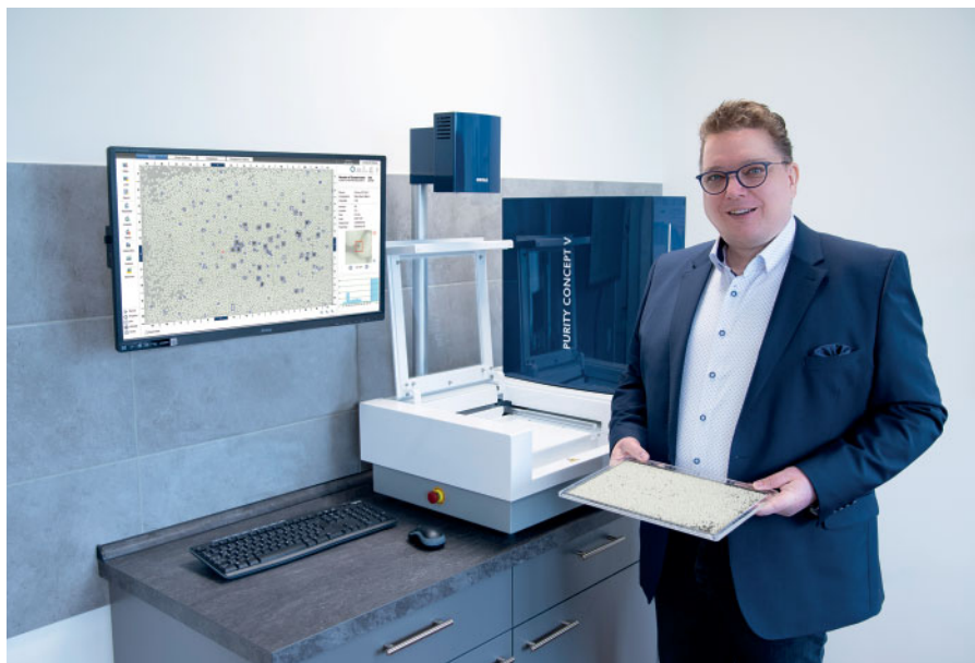
Picture 1: Hilger Groß, Head of Sales and QM at SORTCO, presents the PURITY CONCEPT V from SIKORA for inspection and analysis of plastic pellets
