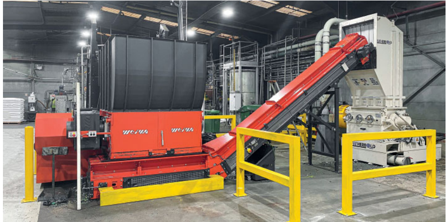
Two-stage shredding solution with WEIMA shredder and Neue Herbold granulator
