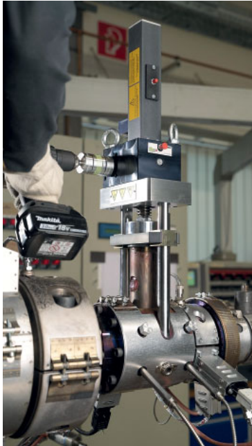
The screen changer is safe to operate manually. To simplify the process, for example, a cordless screwdriver can be used (Photo: W. MÜLLER)
