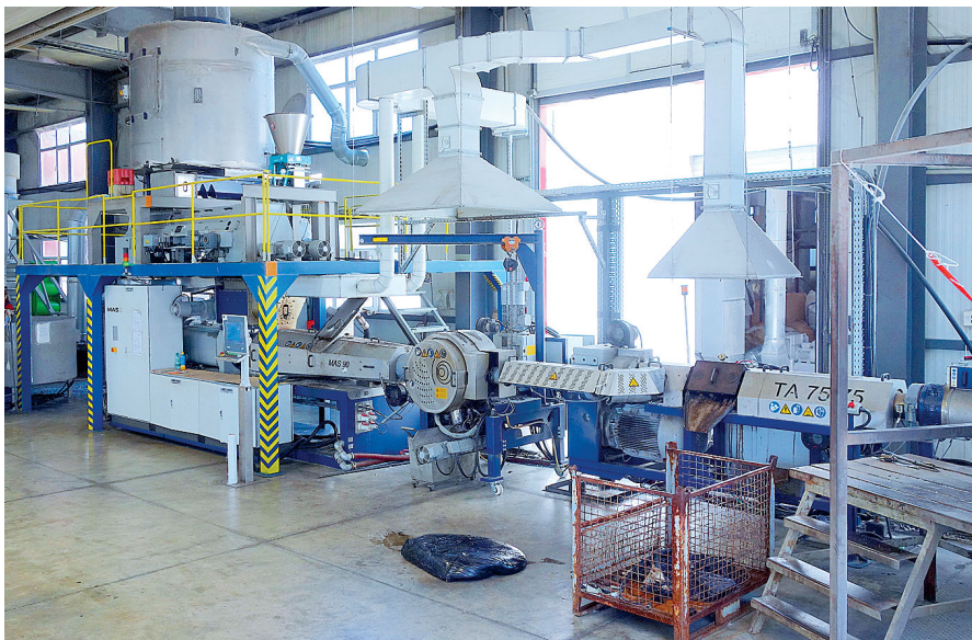
Picture 5: The processed film flakes are pre-dried by the washer to the MAS cascade extrusion line, consisting of conical twin-screw extruder, fed filter and single-screw degassing extruder
