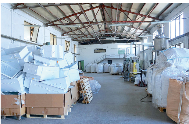
Picture 2: The Kaskada business model is focussed on segregated industrial plastic waste, here at the example of ABS-components from the neighboring refrigerator factory
