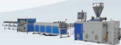
PVC一模双出、四出电工套管挤出生产线 PVC Pipe Two Stand and Four Stand Electric Protection Pipe Extrusion Line
