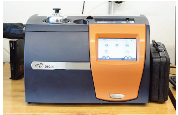
TA Instruments DSC-25 Differential Scanning Calorimeter
